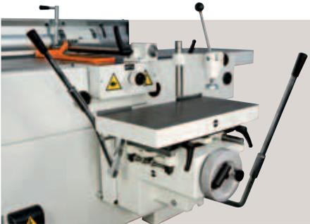
**Mortiser:** It has a cast-iron table of large size that can be easily handled in horizontal, vertical and cross movements with wide strokes in order to increase the performances.
